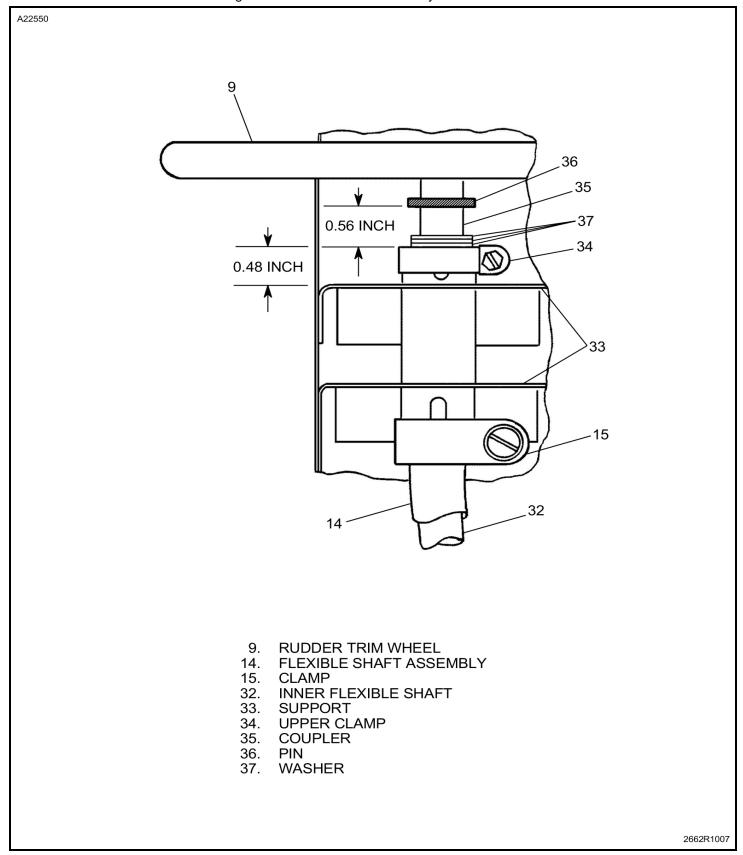
Figure 201: Sheet 2: Rudder Trim System Installation
